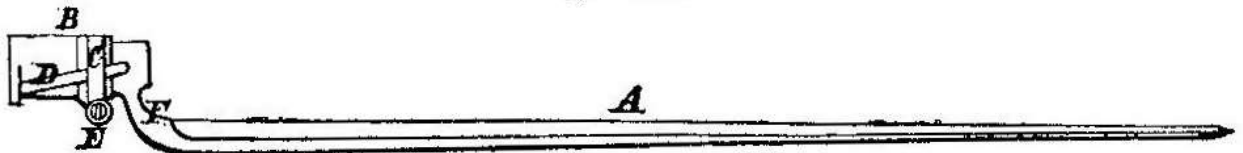
A. Blade. B. Socket. C. Rotating Ring. D. Cut-out. E. Screw. F. Neck.
