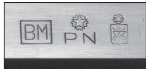
These are the three standard stampings on every Italian-made black powder revolver, pistol, rifle and shotgun. From left to right: year of manufacture, Gardone V.T. black powder proof house stamping, and Gardone proof house stamping. The year of manufacture is?
