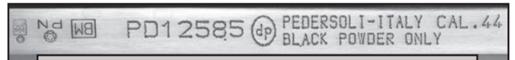
The barrel pictured is a perfect example as it bears all of the Italian proof marks described. This is from a Deluxe engraved Pedersoli Le Page pistol, and all of the stampings are on the underside of the barrel. From left to right (upside down) are the test house and black powder proof house stampings, followed by a boxed BM, denoting a manufacturing date of 1999, then the gun's serial number, a dp oval manufacturer's mark, as well as the PEDERSOLI name, pistol caliber and notification that the gun is for black powder only. This warning appears on the barrel or barrel lug of all black powder arms manufactured in Italy.
